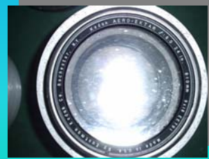
One of the Kodak AERO-EKTAR objectives of the Bamberg Astrogroph used for the Southern Survey.
